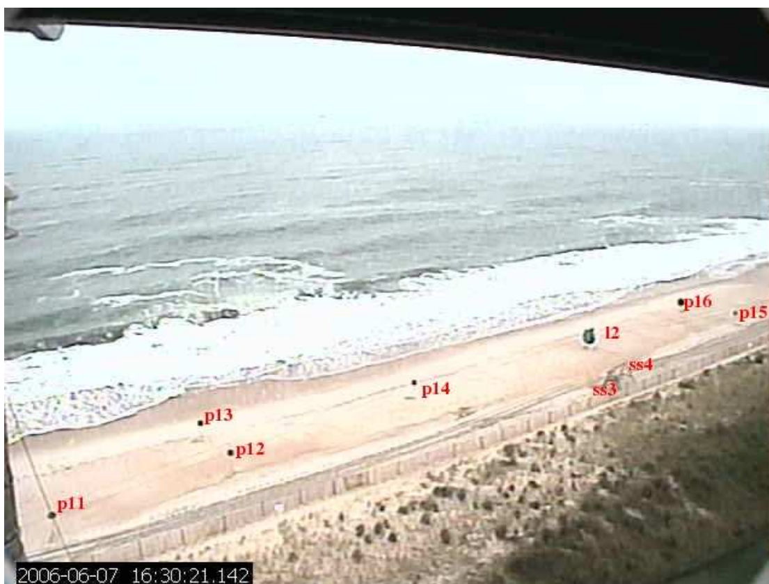
Figure B.25: Camera 4 snapshot with GCPs labeled.
