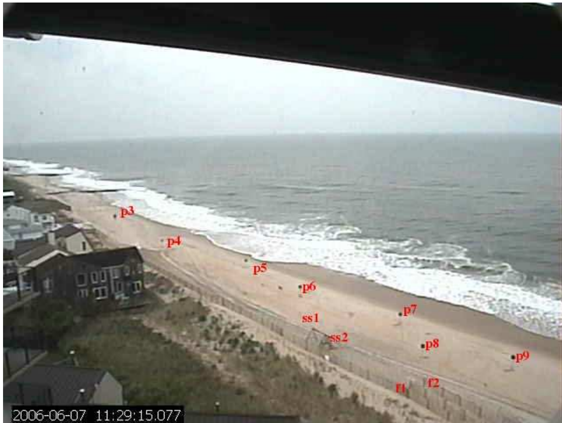
Figure B.23: Camera 2 snapshot with GCPs labeled.
