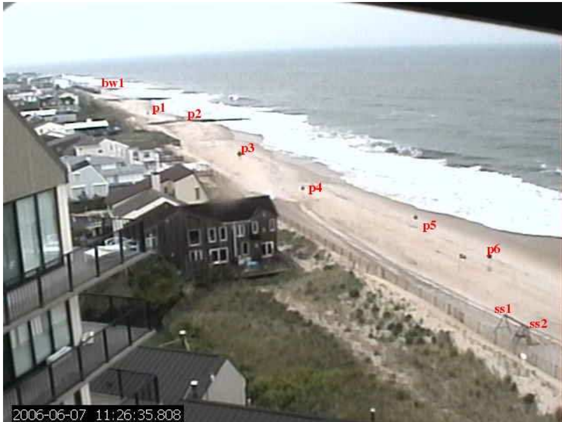
Figure B.22: Camera 1 snapshot with GCPs labeled.
