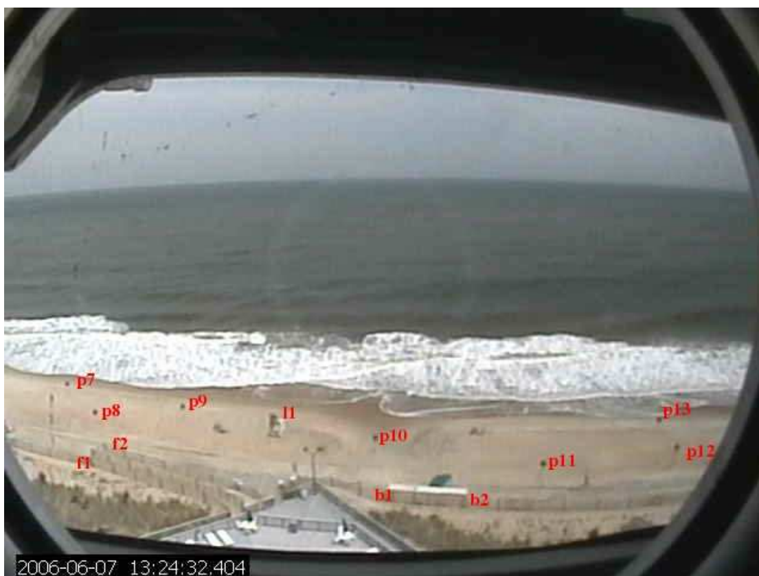
Figure B.24: Camera 3 snapshot with GCPs labeled.
