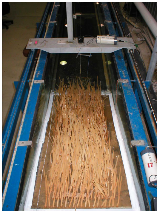
Figure 3.4 Picture of Model Eelgrass Bed in Flume Facing Wave Maker
