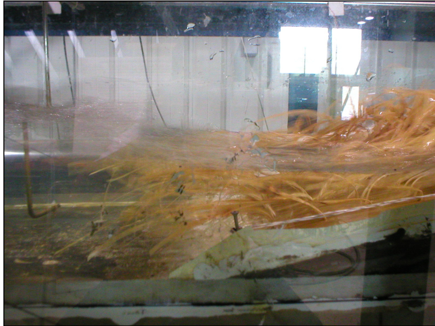
Figure B5 Plan View of Flume at Gage 6 During Case 6 With Plants Run
