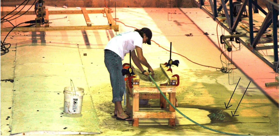
Figure 3.3: This photograph shows the sand washing process. The arrows point to the fines that had passed through the sieve.
