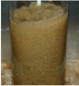
Figure 2.15: This photograph shows the difficulties in suspending sediment at a steady and uniform concentration in a calibration chamber.
