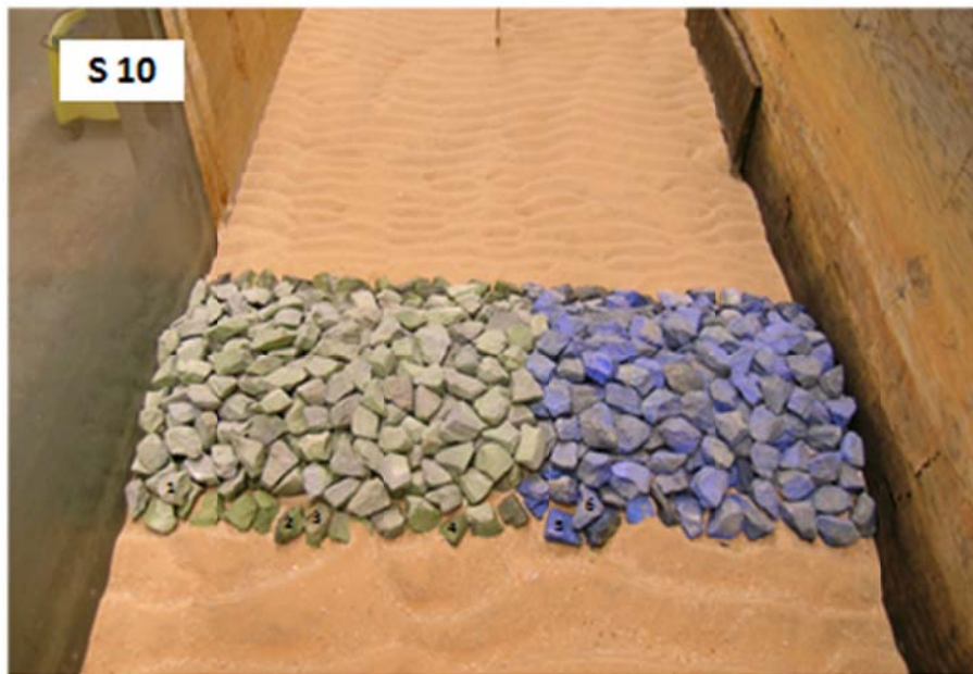
Figure 6-11: Picture of the structure after ten runs in S test (S 10).
