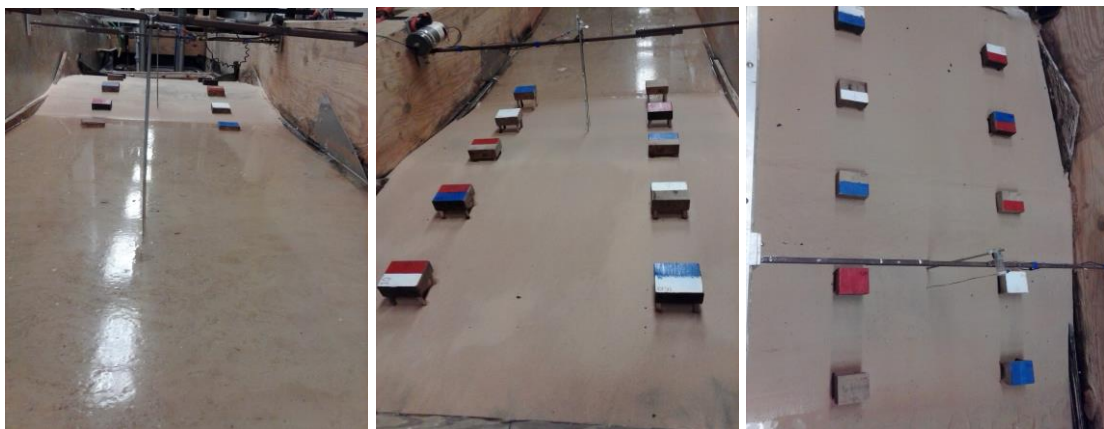
Figure 2.7. Initial block locations before tests: HG with block 1 floating and block 2 at floating limit (left), ML (middle), and MS (right).
