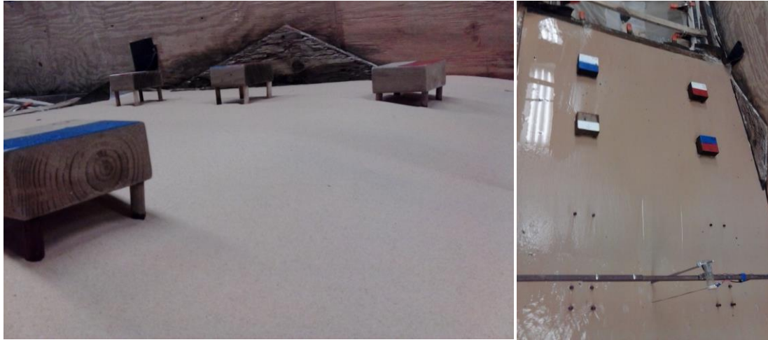
Figure 2.9. Blocks 5 and 6 with clearance decreasing landward and buried rear pilings after run 1 of test LS (left) and pilings of blocks 5 and 6 after test LS (right).
