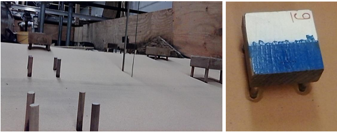
Figure 2.8. Block zone after test LL with blocks 1, 2, and 3 removed (left) and local scour depth (right).
