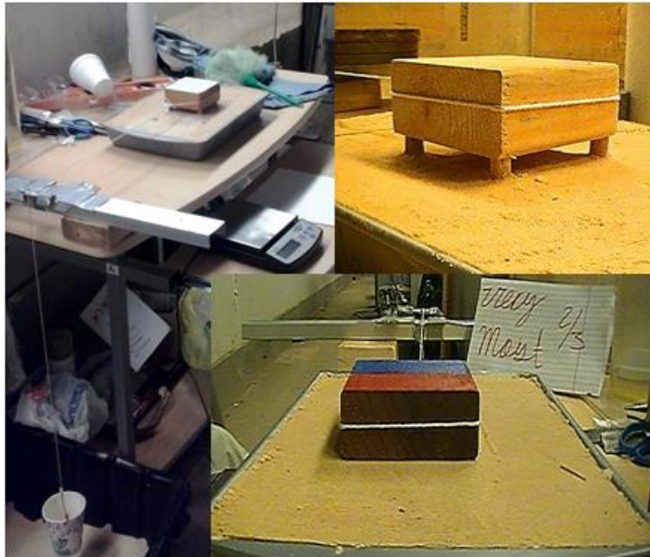
Figure 2.3. Pulling apparatus used to estimate the friction coefficient.
