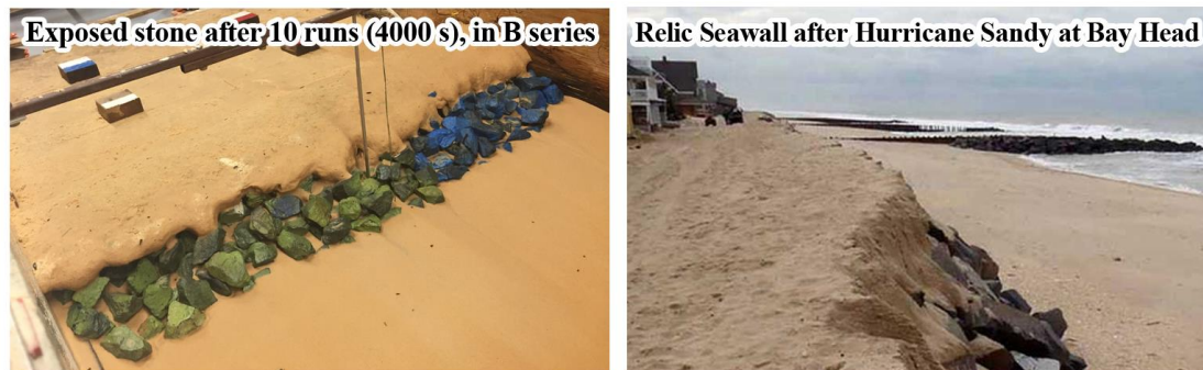
Figure 3.6: Partially exposed stone due to dune erosion after 10 runs (4,000 s) in series B and after Hurricane Sandy at Bay Head (Irish et al 2013)
