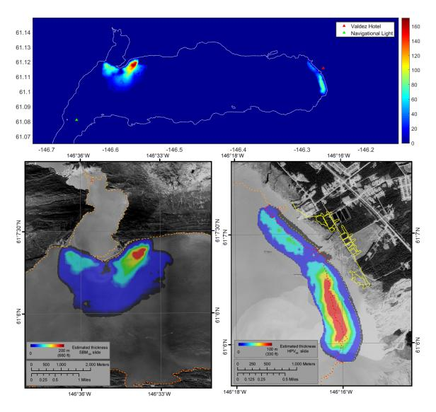
Figure 42: Upper panel: schematic view of Port Valdez with location the two slides; Lower panel: thickness of SBM slide (left) and HPV slide (right). (From Nicolsky et al., 2013)
