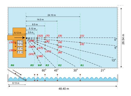
Figure 35: Wave gauge locations in the wave basin.
