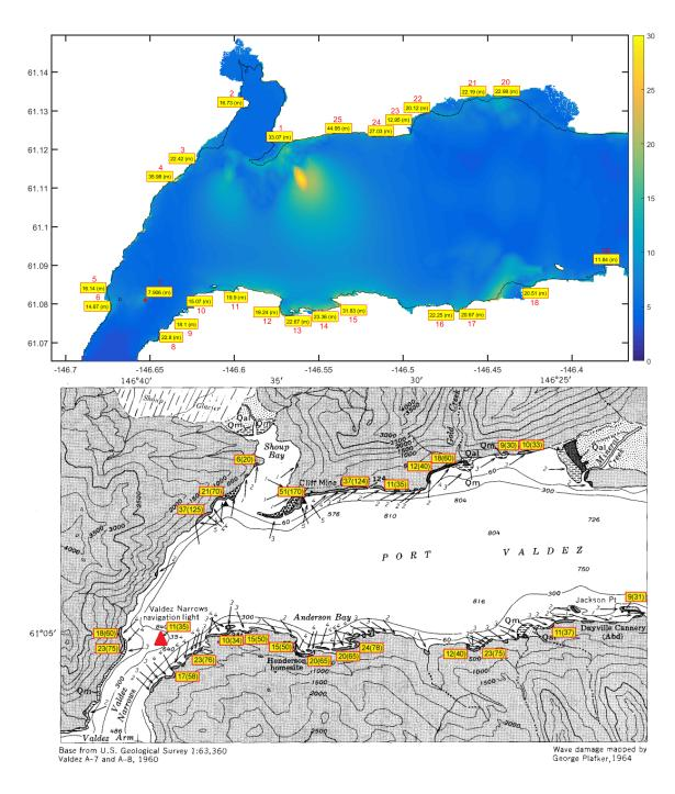
Figure 49: Comparison of maximum runup between computation and observation in Port Valdez..
