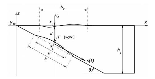
Figure 2: Sketch of main parameters for 2D landslide benchmark. [from Grilli and Watts, 2005].
