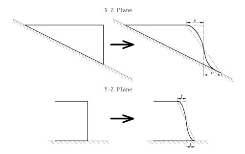
Figure 20: Smoothness of triangular block
