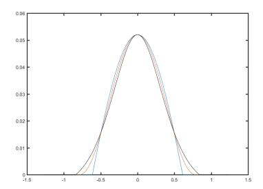
Figure 5: Slide cross-section geometry for 2D model. Blue line represents Gaussian shape with  $\varepsilon=0.75$ , black line represents the one with  $\varepsilon=0.1$  and red line represents Cosine shape.
