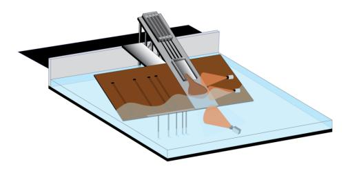
Figure 34: Landslide tsunami generator setup
