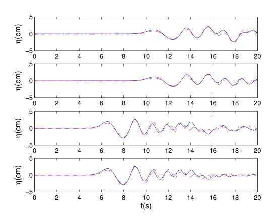
Figure 37: Benchmark 6: Model-data comparisons of tsunami waves for stations 1 to 4.
