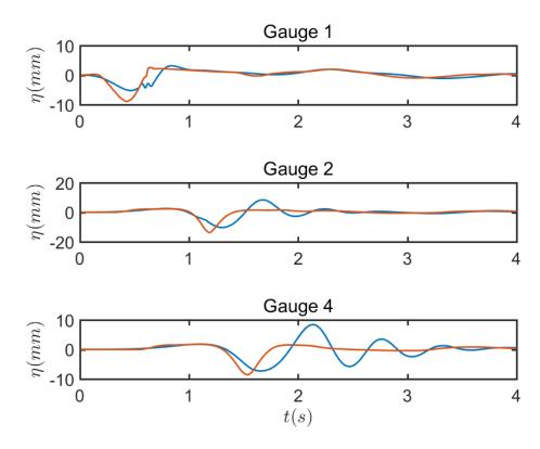
Figure 18: Comparison of results for case  $d=120\,\mathrm{mm}$  between numerical solution with and without non-hydrostatic pressure. Blue lines represent numerical solution with non-hydrostatic pressure and red lines represent the solution without non-hydrostatic pressure.
