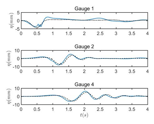
Figure 13: Benchmark 2: Comparison of surface elevation between numerical results of the case  $d=149~\mathrm{mm}$  from NHWAVE and experimental data at locations of  $(\mathbf{x},\mathbf{y})=(0.877,0), (1.469,350), (1.919,500)$  in meters. Solid blue lines represent numerical results and dashed black lines represent experimental data.
