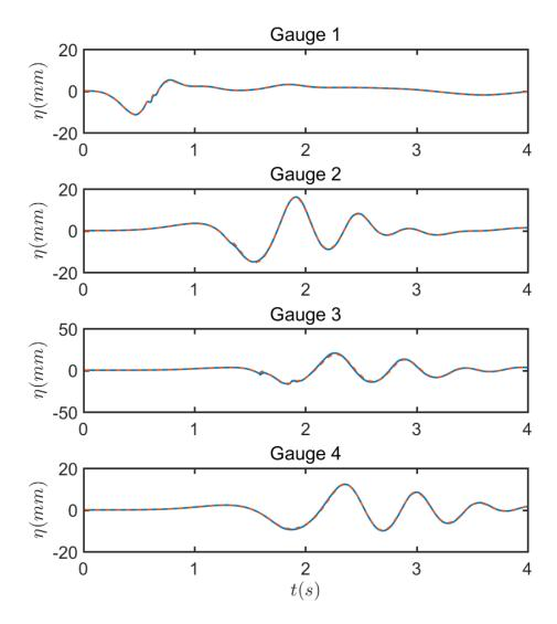
Figure 15: Comparison of results for case d=61 mm between numerical solution and analytical solution for  $\mathrm{d}h/\mathrm{d}t$  and  $\mathrm{d}^2h/\mathrm{d}t^2$ . Solid blue lines represent numerical solution and dashed red lines represent analytical solution.
