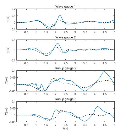
Figure 21: Benchmark 3: Comparison of surface elevation and runup at 4 gauges for case  $\Delta=0.10$  m between numerical results and experimental data. Solid blue lines represent numerical results and dashed black lines represent experimental data.
