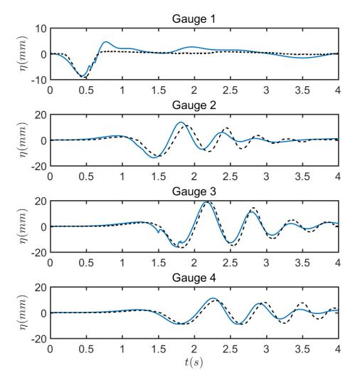
Figure 9: Benchmark 2: Comparison of surface elevation between numerical results of the case d=80 mm from NHWAVE and experimental data at locations of (x,y)=(0.617,0), (1.469,350), (1.929,0), (1.919,500) in meters. Solid blue lines represent numerical results and dashed black lines represent experimental data.
