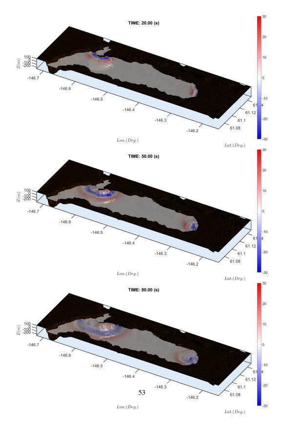
Figure 45: Wave elevation in Port Valdez at 20, 50 and  $80 \ s$ .
