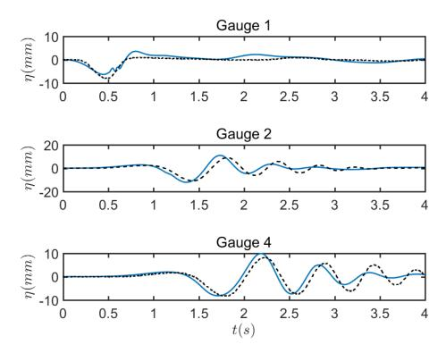
Figure 10: Benchmark 2: Comparison of surface elevation between numerical results of the case  $d=100~\mathrm{mm}$  from NHWAVE and experimental data at locations of (x,y)=(0.696,0), (1.469,350), (1.919,500) in meters. Solid blue lines represent numerical results and dashed black lines represent experimental data.
