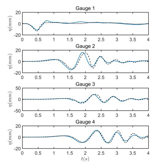
Figure 8: Benchmark 2: Comparison of surface elevation between numerical results of the case d=61 mm from NHWAVE and experimental data at locations of  $(\mathbf{x},\mathbf{y})=(0.551,0), (1.469,350), (1.929,0), (1.919,500)$  in meters. Solid blue lines represent numerical results and dashed black lines represent experimental data.
