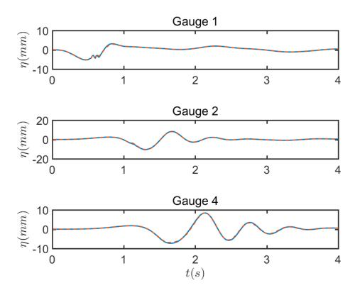
Figure 16: Comparison of results for case d=120 mm between numerical solution and analytical solution for  $\mathrm{d}h/\mathrm{d}t$  and  $\mathrm{d}^2h/\mathrm{d}t^2$ . Solid blue lines represent numerical solution and dashed red lines represent analytical solution.
