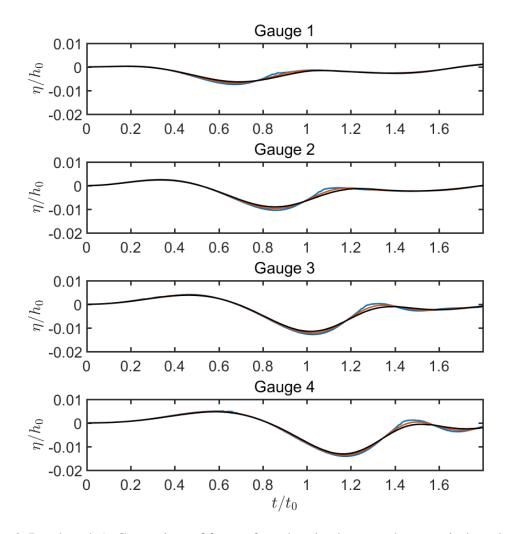
Figure 6: Benchmark 1: Comparison of free surface elevation between the numerical results with three types of model geometry. Blue line represents Gaussian shape with  $\varepsilon=0.75$ , black line represents the one with  $\varepsilon=0.1$  and red line represents Cosine shape.
