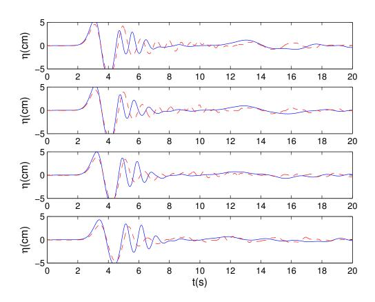
Figure 40: Benchmark 6: Model-data comparisons of tsunami waves for stations 13 to 16.
