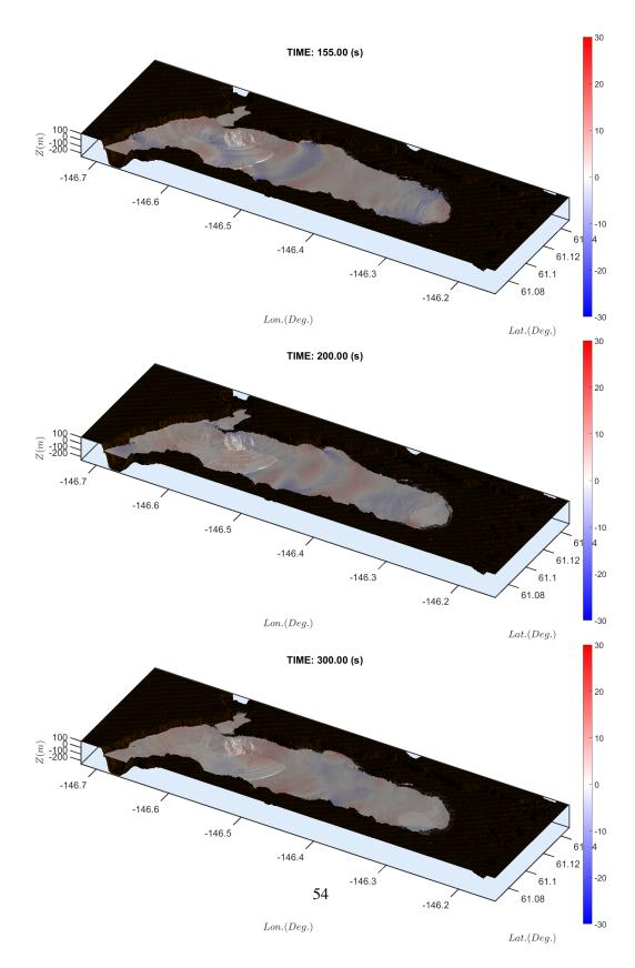
Figure 46: Wave elevation in Port Valdez at 155, 200 and  $300 \ s$ .
