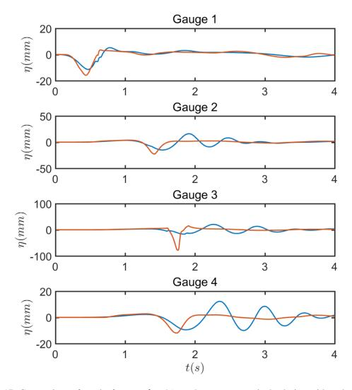
Figure 17: Comparison of results for case  $d=61\,\mathrm{mm}$  between numerical solution with and without non-hydrostatic pressure. Blue lines represent numerical solution with non-hydrostatic pressure and red lines represent the solution without non-hydrostatic pressure.
