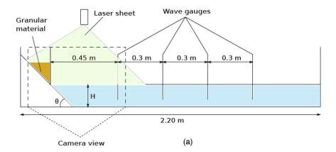
Figure 30: Set-up for laboratory experiments of tsunami generation by subaerial slides made of glass beads performed in IRPHE's precision tank of (useful) length l=2.20 m, width w=0.2 m, and water depth H=0.150 m. Upon release, beads are moving down a slope of  $\theta=45^{\circ}$ . The slide shape and water motion are recorded with high speed video camera and laser PIV, respectively. Surface elevations are recorded at 4 wave gages (WG1, WG2, WG3, WG4) marked on the figure.
