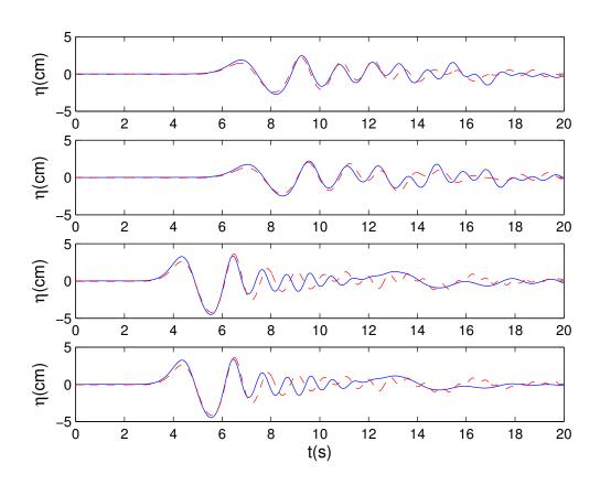
Figure 38: Benchmark 6: Model-data comparisons of tsunami waves for stations 5 to 8.
