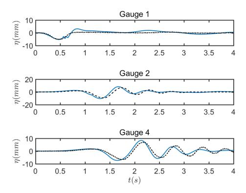
Figure 11: Benchmark 2: Comparison of surface elevation between numerical results of the case  $d=120~\mathrm{mm}$  from NHWAVE and experimental data at locations of  $(\mathrm{x,y})=(0.763,0), (1.469,350), (1.919,500)$  in meters. Solid blue lines represent numerical results and dashed black lines represent experimental data.
