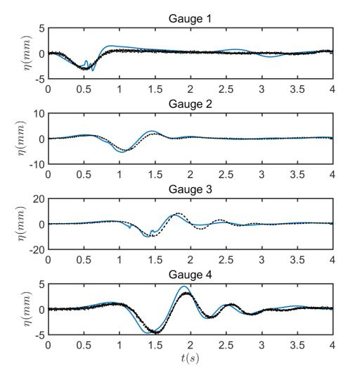
Figure 14: Benchmark 2: Comparison of surface elevation between numerical results of the case  $d=189~\mathrm{mm}$  from NHWAVE and experimental data at locations of (x,y)=(1.017,0), (1.469,350), (1.929,0), (1.919,500) in meters. Solid blue lines represent numerical results and dashed black lines represent experimental data.
