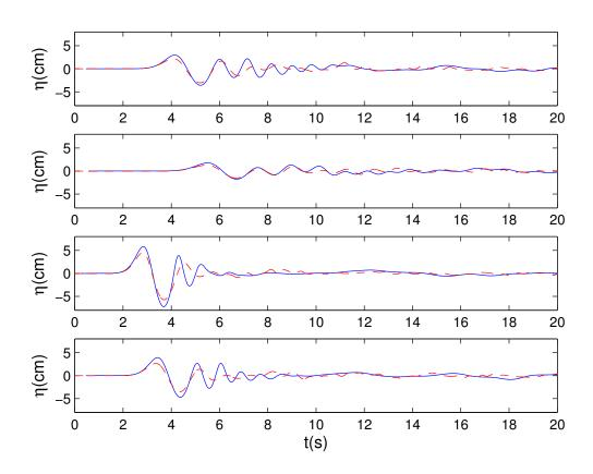
Figure 41: Benchmark 6: Model-data comparisons of tsunami waves for stations 17 to 20.
