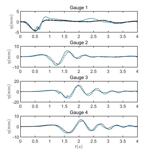
Figure 12: Benchmark 2: Comparison of surface elevation between numerical results of the case  $d=140~\mathrm{mm}$  from NHWAVE and experimental data at locations of (x,y)= (0.846,0), (1.469,350), (1.929,0), (1.919,500) in meters. Solid blue lines represent numerical results and dashed black lines represent experimental data.
