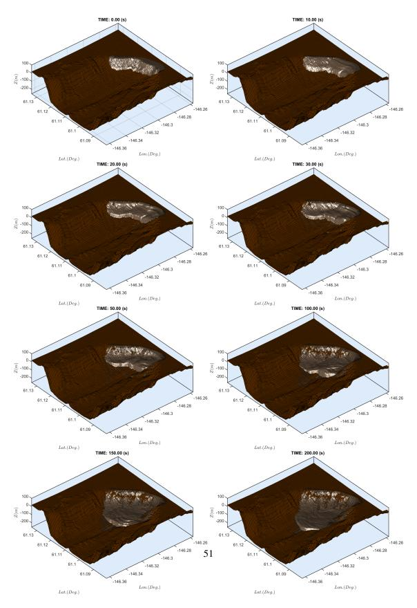
Figure 43: Motion of HPV slide at 0, 10, 20, 30, 50, 100, 150 and 200 s.
