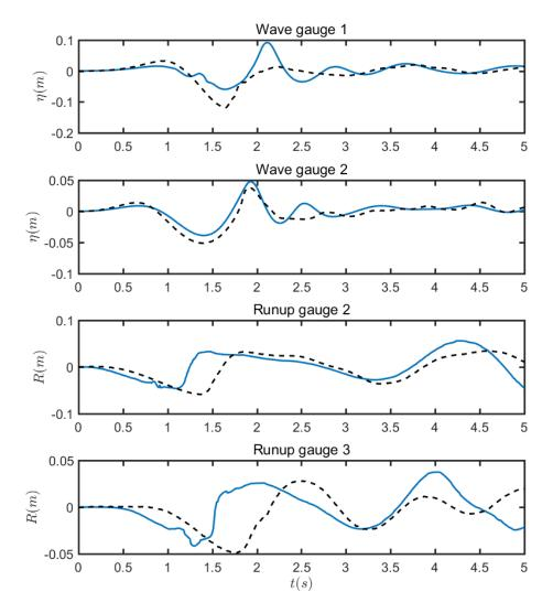
Figure 22: Benchmark 3: Comparison of surface elevation and runup at 4 gauges for case  $\Delta=-0.025$  m between numerical results and experimental data. Solid blue lines represent numerical results and dashed black lines represent experimental data.
