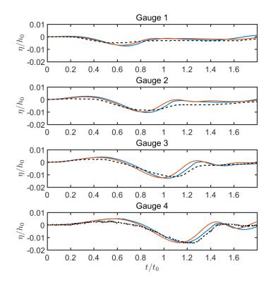
Figure 3: Benchmark 1: Comparison of surface elevations obtained from NHWAVE with solid slide motion, with BEM results (Grilli and Watts 2005) and experimental data at locations of x=1.234, 1.549, 1.864, 2.179 m. Solid blue lines represent NHWAVE results, solid red lines represent BEM results and dashed black lines represent experimental data.
