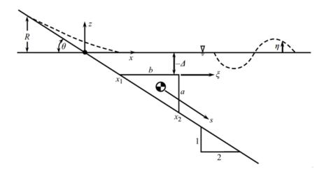
Figure 19: Sketch of main parameters for 3D subaerial/submarine triangular landslide benchmark.(From Liu et al., 2005)
