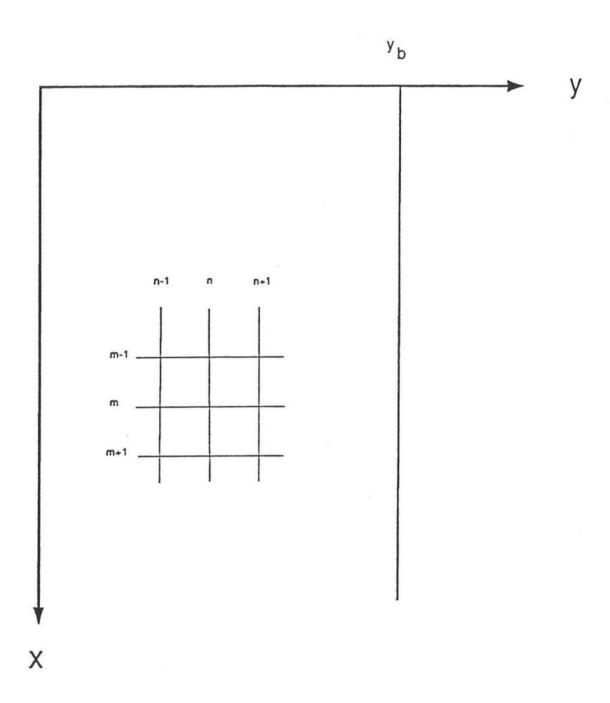
Figure 1: A sketch of the computational domain  $(x > 0, 0 < y < y_b)$  and the analytical domain  $(x > 0, y > y_b)$ . A piece of the computational mesh is also shown.
