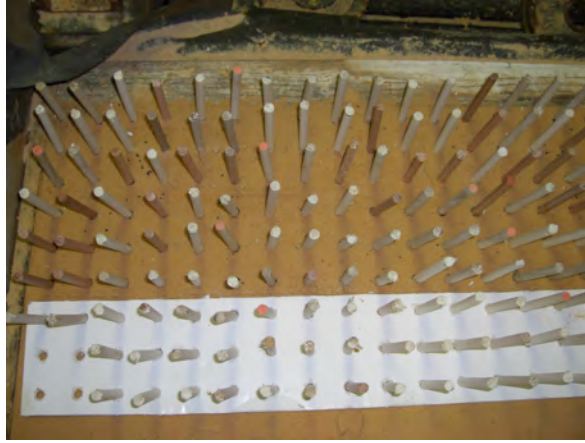
Figure 2.8: Template to create a uniform vegetation field throughout the experiment.
