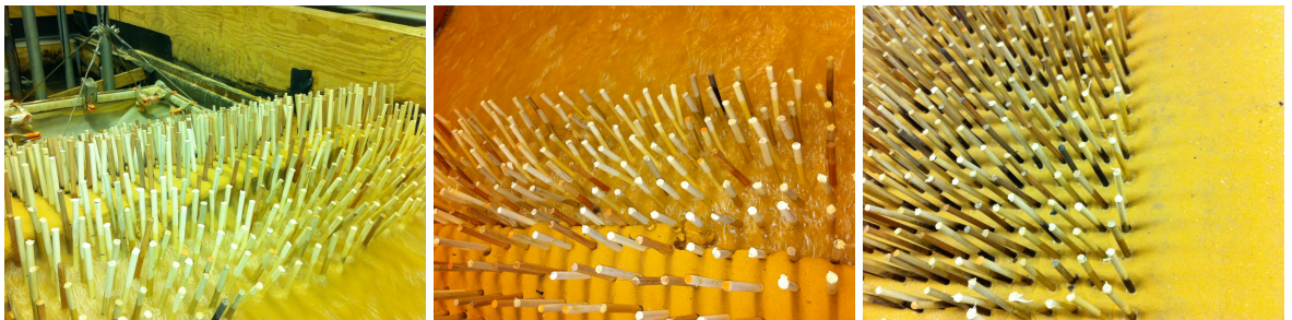
Figure 3.9: Photos taken during the HW (left and middle) and LW (right) tests illustrating scarping and slumping processes for the high dune test series and the hump formed during the low dune test with the wide vegetation.
