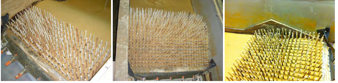
Figure 2.6: Vegetation configurations for the HN (left), HW (middle), and LW (right) test under initial conditions. The HW and LW tests show the same setup of the vegetation field.
