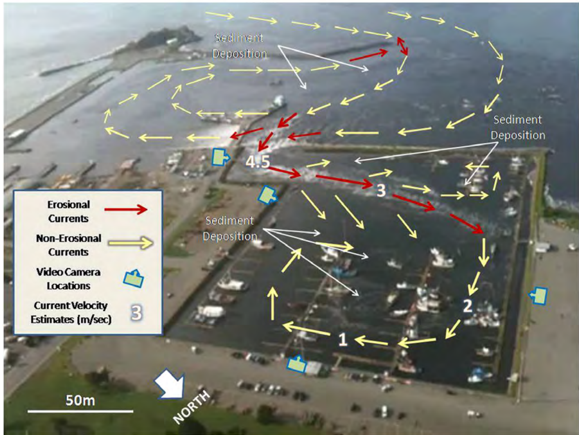
Figure 4.16: Tsunami flow-regime map for Crescent City Harbor. Current directions and velocities, and areas of sediment erosion and deposition are based on observations of the various (30) ground-level and aerial video, pre- and post-tsunami bathymetry, and sediment analyses (Figure taken from Wilson et al., 2012, Figure 5)
