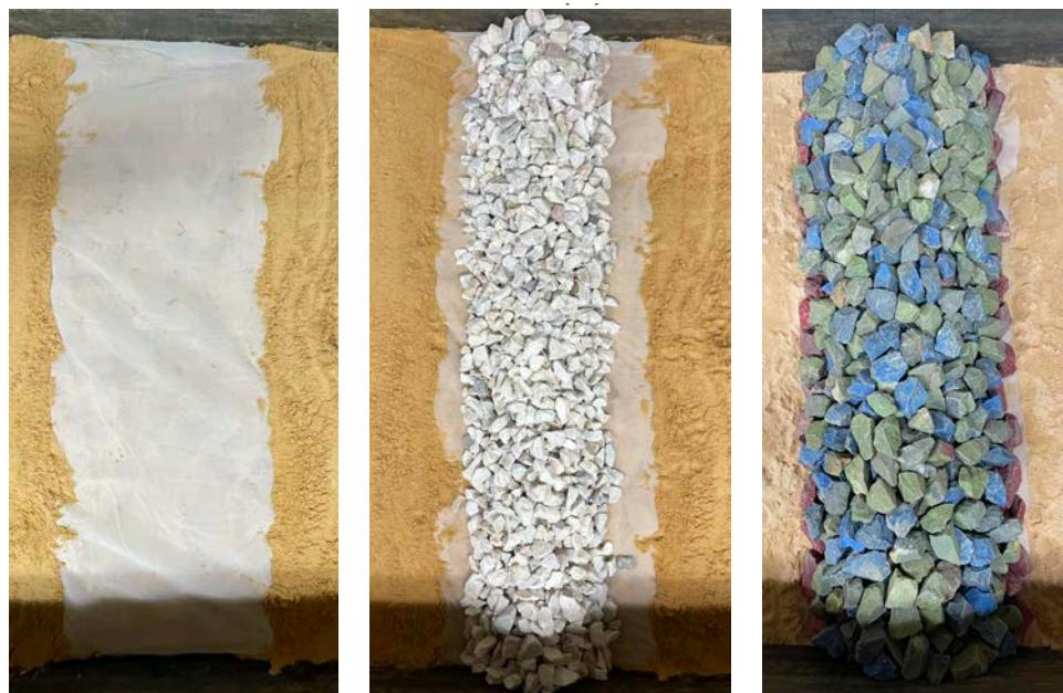
**Figure 2.3** Initial rubble mound profile in D test with photos showing the placement of filter, white core stones, and double-layer (blue and green)
